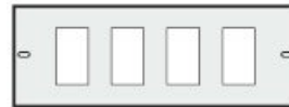
4-RJ45/4 4 off RJ45 Cutouts (Cutout size 37mm x 22mm, other punchings available)
